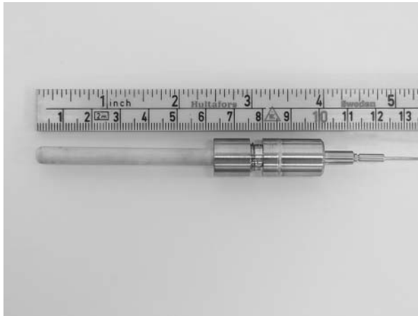
11.17 Prototype Fe/Fe 3 O 4 reference electrode
