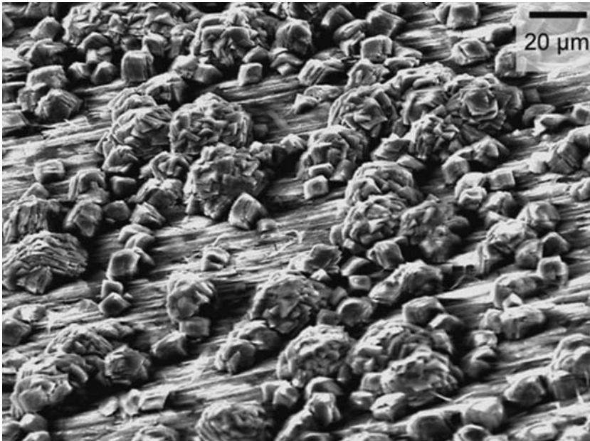
9.9 SEM observation of carbon steel surface corroded in granitic solution without clay at 90°C after 700 h
